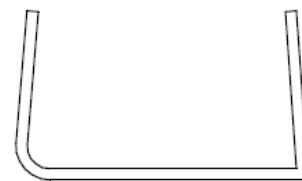
Die 1505 — 24mm Capping Section
