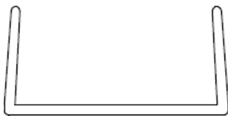
Die 1557 — 22mm Capping Section
