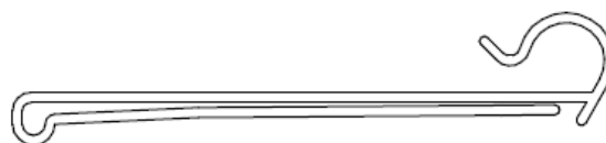
Die 1707 — 39mm Swing Ticket (For 4.5mm Wire)
