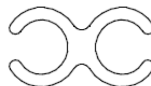
Die 1578 — Figure of 8 Channel
